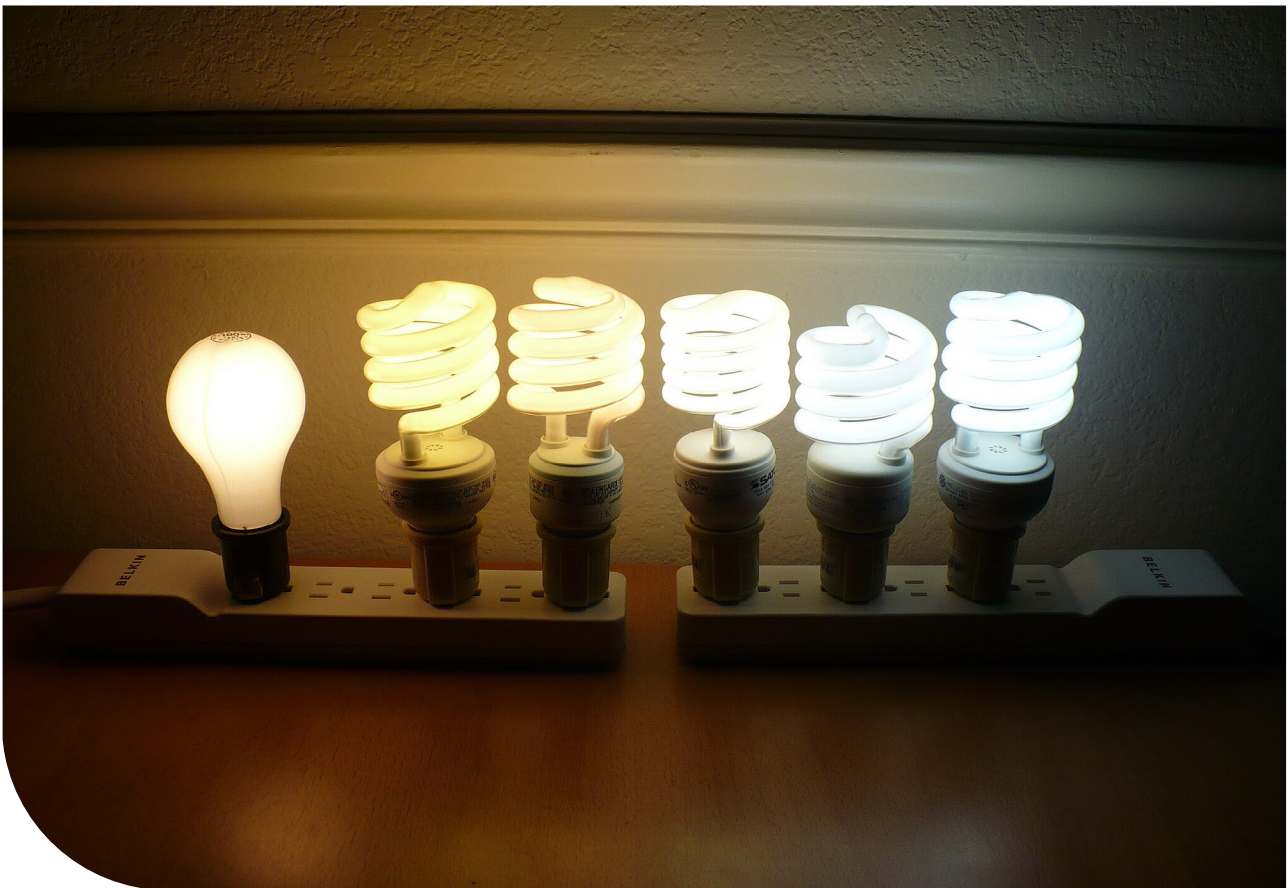
Comparison of correlated colour temperature (CCT) of five lamps (indoor compact fluorescent light bulbs). From left (warmer yellow) to right (cooler blue): 2700K, 3500K, 4100K, 5500K, 6500K. The warmer yellow lower CCT light, is suggested for exterior lighting due to the lower amount of blue light – known to be harmful to many nocturnal species. Source: User: Splarka, Public domain, via Wikimedia Commons, https://commons.wikimedia.org/wiki/File:Color_temperature_comparison_of_5_CFLs.jpg
