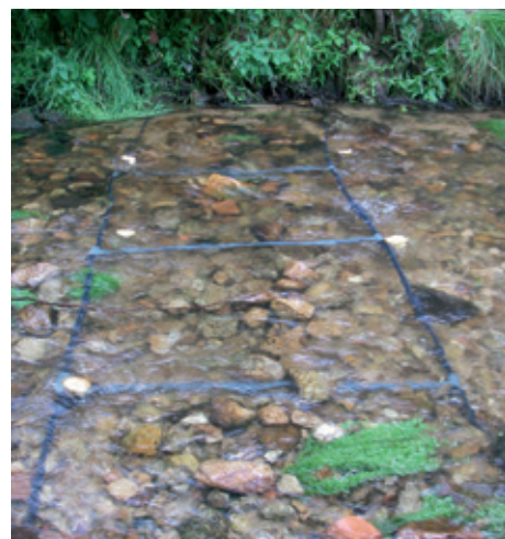
Figure 5: Left: set-up diagram of culvert OH 448 with fixed RFID antennae. Boxes A1 and A2 represent the fixed RFID antennae placed upstream of the culvert. Right: picture of an antenna set up in the Durolle.
