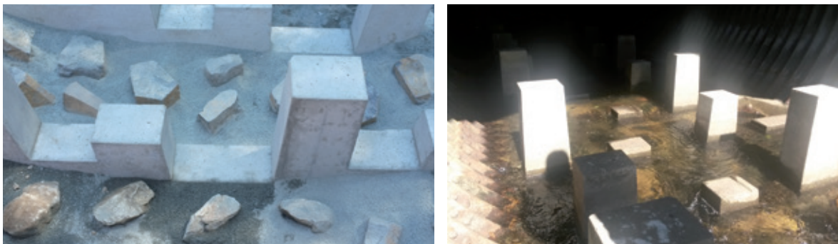
Figure 3: Unique hydraulic system consisting of a rough-textured base plate and prefabricated flow-breakers.
