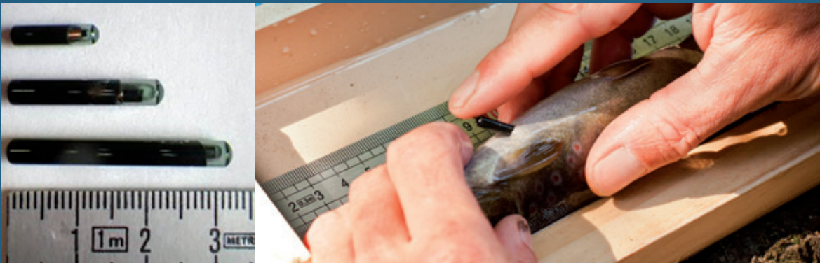
Illustration 1: Various sizes of transponders (left) that can be used for tagging trout (right).
