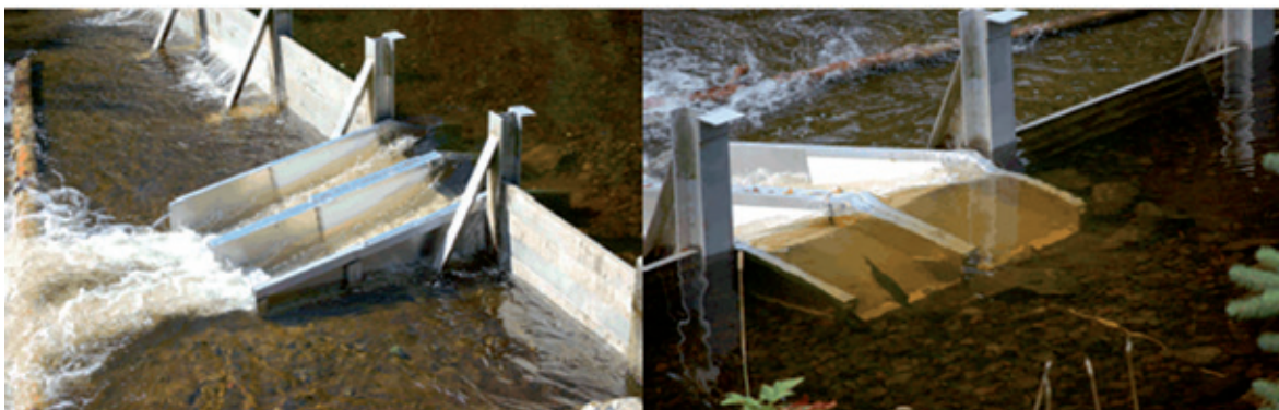
Figure 39: Example of a resistivity counter used in a river (Diagram: Loughs Agency (2016); Photo: InStream Fisheries Research).
