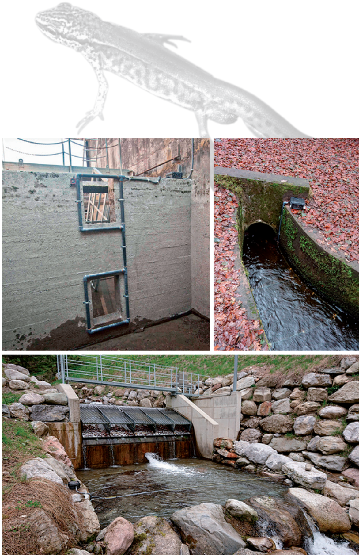
Figure 31 : Examples of designs of RFID antennae set up in various habitats (SCIMABIO Interface studies, 2019-2021)
