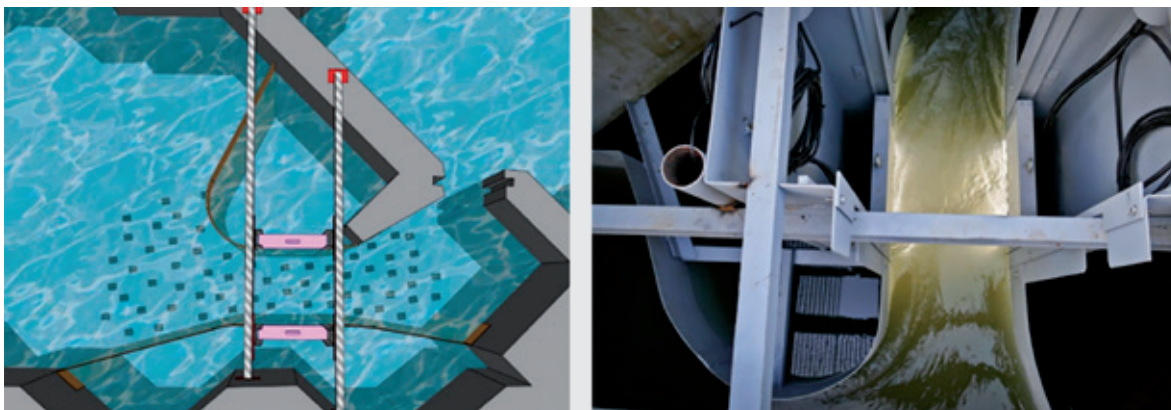
Figure 35 : Set-up of a video counting system in an existing fish pass. Utilisation of solid deflectors to ensure the quality of the hydraulic intersection.
