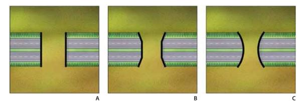
Figure 1.2. Alternative plans for ecoduct designs.
