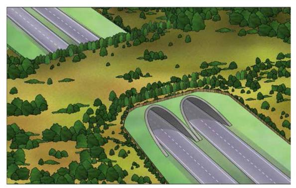
Figure 1.1. Diagram of a ecoduct.
