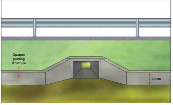
Figure 11.1. Diagram of an amphibian crossing.
