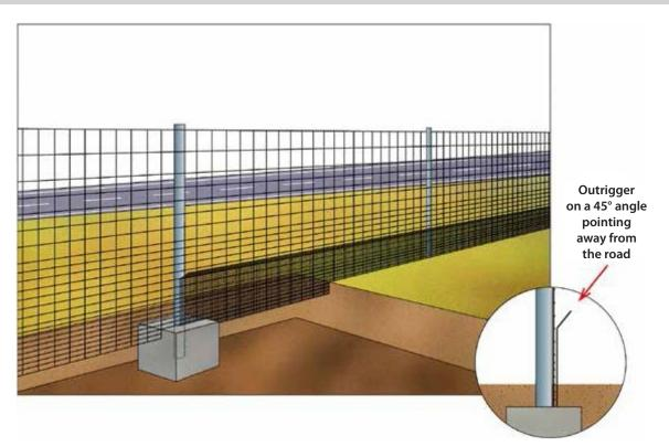
Figure 14.1. Diagram of reinforcement mesh, attached to the base of a fence for large mammals in order to prevent breaches by small vertebrates.
