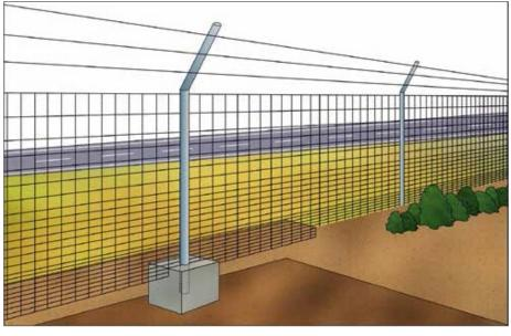
Figure 13.4. A fence can be extended upwards using outrigger poles angled away from the road, topped with galvanized barbed wire. The base of the fence should be buried.
