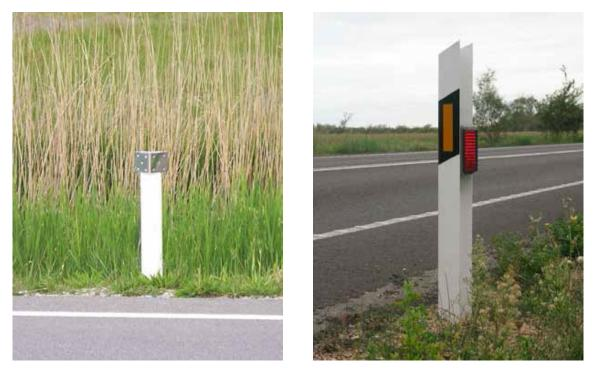
Figure 18.2. Various models of reflectors are available to project headlight beams into the natural surroundings of roads. These systems require frequent maintenance and have short-term effectiveness. Photos: C. Rosell.
