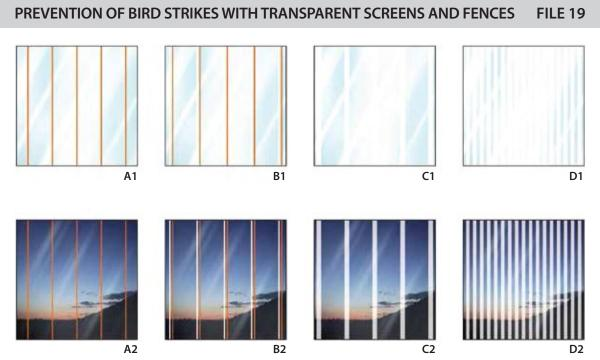
Figure 19.1. Diagram showing various types of vertical stripes for roadside screens. The colours must ensure maximum contrast with the background during the peak periods of bird movement. The combination of orange and white (B1 and B2) yields the best results for different situations.
