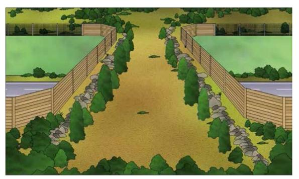
Figure 2.1. Diagram of an wildlife overpass.
