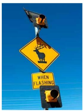
Figure 17.3. Flashing warning sign activated by animal detection sensors (ADS). Photo: C. Rosell.
