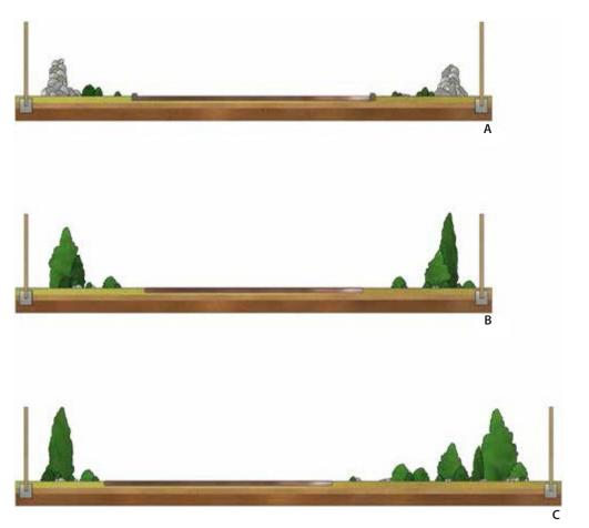
Figure 3.2. Section of tracks and verges on a multi-use overpass. The track should be set in the central section (A and B) or, if the structure is wide enough, along one side (C). In the case of overpasses in arid zones, the vegetation can be replaced by low dry stone walls or rows of stones to guide the wildlife movement and provide shelter for small animals (A).
