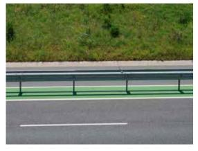
Figure 16.2. Unvegetated lane separation median strips. This may be appropriate on road sections where the proliferation of voles and other prey attract raptors and carnivores, increasing the roadkilling hazard. Photo: C. Rosell.
