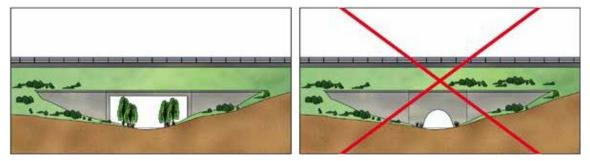
Figure 5.2. Frame bridges and archs are less suitable than viaducts for roads that cross a river valley. If such structures are used, their size should permit the continuity of the riparian vegetation.
