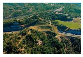
Figure 1.4. The ecoduct surface and access zones should have similar topographic profiles to the surrounding landscape. Photo: Minuartia.
