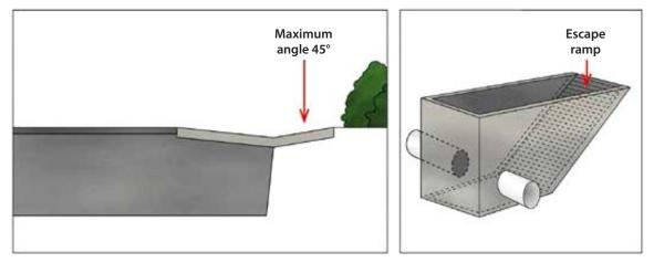
Figure 20.1. Diagram of an angled kerb and an exit ramp from a manhole or similar drainage infrastructure.
