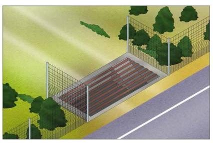
Figure 15.6 Diagram of a cattle grid for ungulates, with an interior escape ramp for animals that might accidentally fall into the trench beneath.
