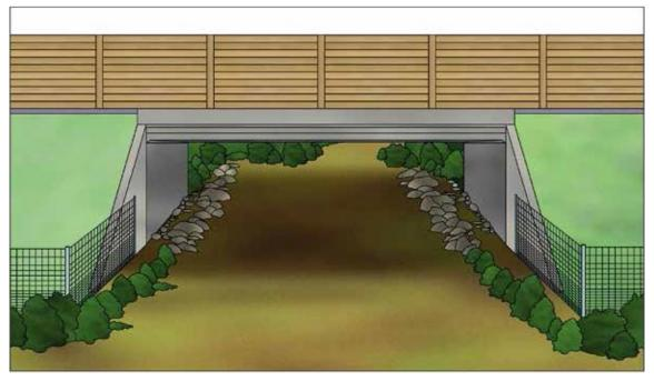
Figure 6.1. Diagram of a large mammal underpass.
